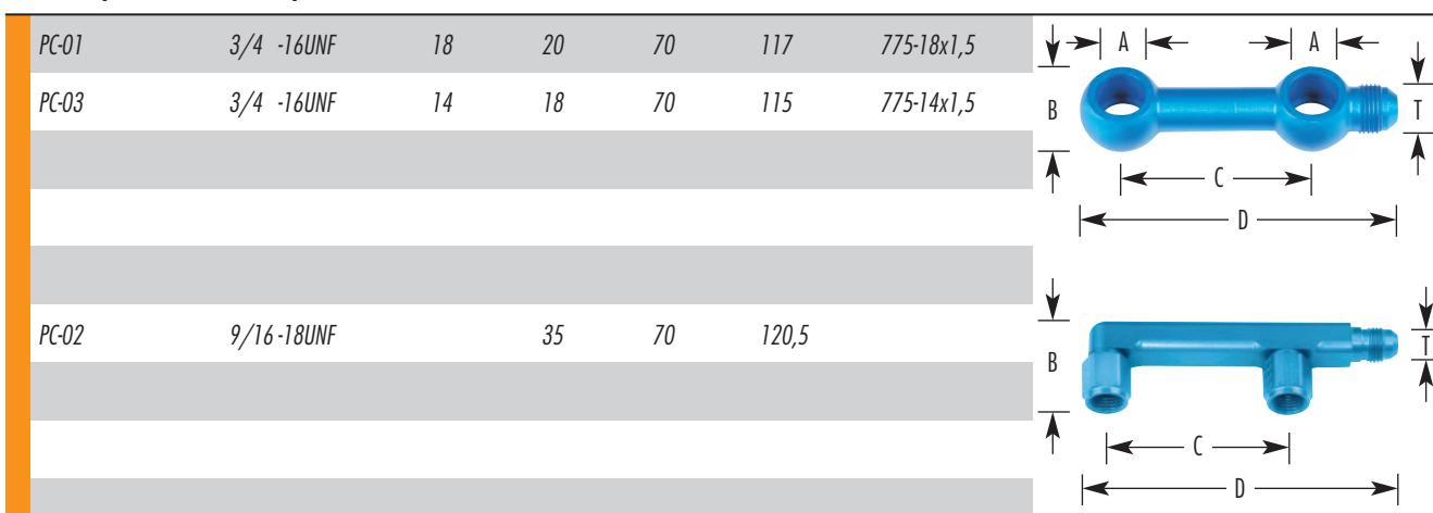
The technical drawings illustrate three types of pump connectors.
